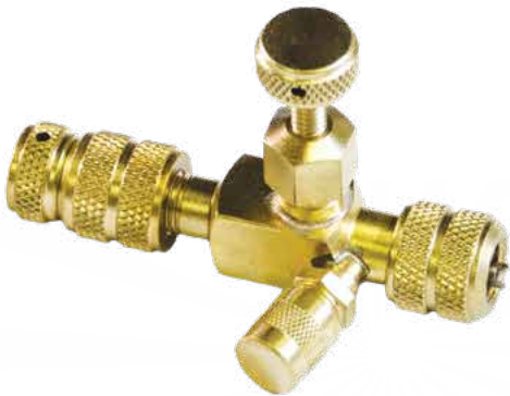
PART# CD3090 PKG QTY: 1 Tube piercing attachment punches a hole in copper tubing through a V-Series fitting for the installation of a core without loss of refrigerant
